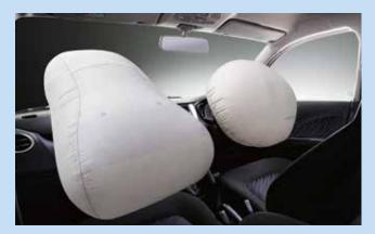
Front airbags mitigate the impact to driver and front passenger in the event of a frontal collision.
