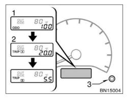
This meter displays the odometer and two trip meters when the ignition switch is on.
