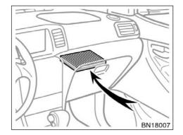
The air conditioning filter is behind the glove box.
