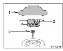
When storing the spare tire, put it in place with the outer side of the wheel facing up. Then secure the tire by repeating the above removal steps in reverse order to prevent it from flying forward during a collision or sudden braking.
