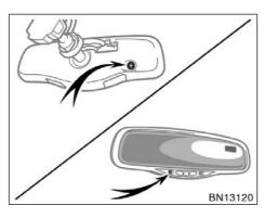
To ensure correct functioning of antiglare mirror sensors located on both sides of the mirror, do not touch or cover the sensors with your finger or a piece of cloth, etc.
