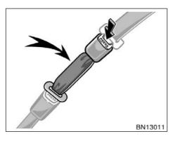
To connect the extender to the seat belt, insert the tab into the seat belt buckle so that the "PRESS" signs on the buckle release buttons of the extender and the seat belt are both facing outward as shown.
