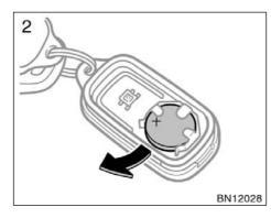
2. Remove the discharged transmitter battery.
