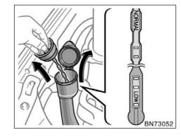
For vehicles sold in the U.S.A.—If any washer does not work, the washer tank may be empty. Check the washer fluid level on the level gauge. If the washer fluid level is at "LOW", add washer fluid.
