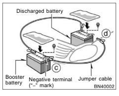
c. Connect the clamp of the negative (black) jumper cable to the negative (-) terminal on the booster battery.
