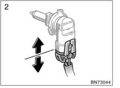
2. Pull the bulb out of the base. Install a new bulb.
