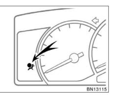
This indicator comes on when the ignition key is turned to the "ON" position. It goes off after about 6 seconds. This means the SRS side airbags and curtain shield airbags are operating properly.
