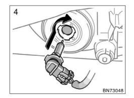
4. Install a new bulb and connector into the mounting hole.
