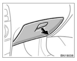
To open the glove box door, pull the lever.
