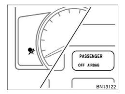
The SRS warning light will come on and front passenger occupant classification indicator light will indicate "OFF" if there is a malfunction in the front passenger occupant classification system.
