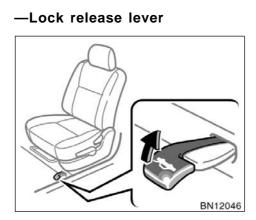
To open the trunk lid from the driver's seat, pull up on the lock release lever.
