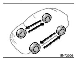
To equalize the wear and help extend tire life, Toyota recommends that you rotate your tires according to the maintenance schedule. (For scheduled maintenance information, please refer to the "Scheduled Maintenance Guide" or "Owner's Manual Supplement".) However, the most appropriate timing for tire rotation may vary according to your driving habits and road surface conditions.
