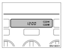
To reset the hour: Push the "H" button. To reset the minutes: Push the "M" button.
