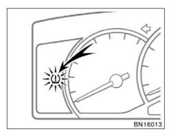
If the low tire pressure warning light does not blink when you push and hold the reset switch, have the low pressure warning system checked at your Toyota dealer.
