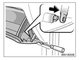
1. Open the glove box. Remove the screw with a Phillips-head screwdriver and slide off the damper as shown.
