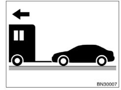
Your vehicle can be dinghy towed (with four wheels on the ground) from the front behind a motorhome.
