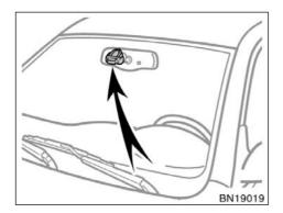
The compass sensor is on the inside rear view mirror.
