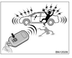
Pushing the "PANIC" switch blows the horn intermittently and flashes the headlights, tail lights, turn signal lights and interior light.
