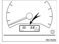
The displayed temperature ranges from  $-30^{\circ}C$  ( $-22^{\circ}F$ ) up to  $50^{\circ}C$  ( $122^{\circ}F$ ).
