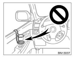
• Do not attach a cup holder or any other device or object on or around the door. When the side airbag inflates, the cup holder or any other device or object will be thrown with great force or the side airbag may not activate correctly, resulting in death or serious injury. Likewise, the driver and front passenger should not hold objects in their arms or on their knees.
