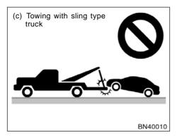
(c) Towing with sling type truck
