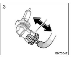
**3. Unplug the connector.** If the connector is tight, wiggle it.
