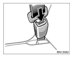
2. To remove the booster seat, press the buckle release button and allow the belt to retract.
