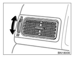
If air flow control is not satisfactory, check the side vents. The side vents may be opened or closed as shown.
